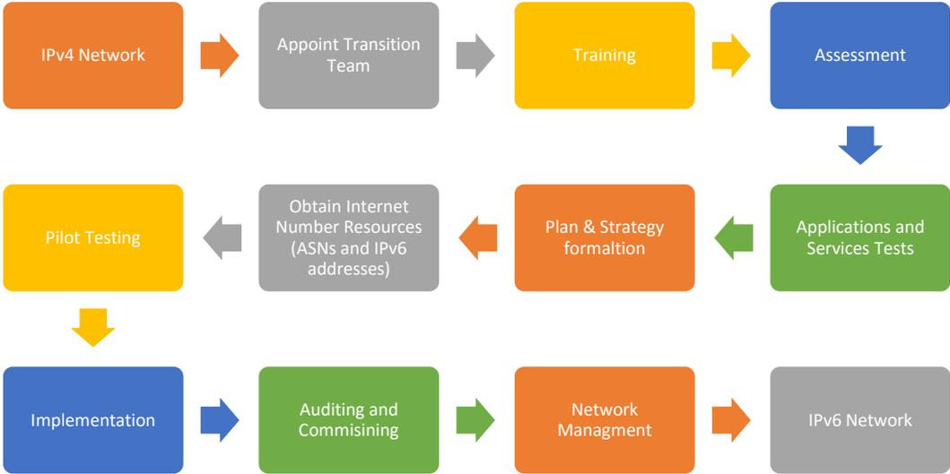
**Figure 1.** Typical phased IPv4 to IPv6 transition approach
