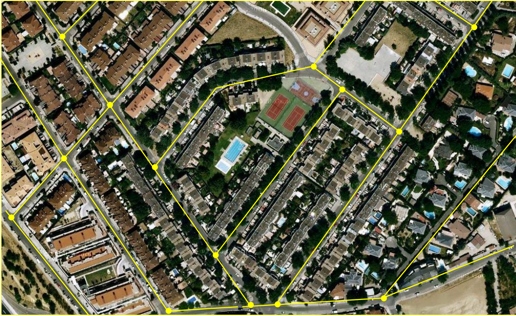
Exhibit 9: Illustrative example of the process to be followed for the dimensioning of the fixed access network. [Source: Axon Consulting]
