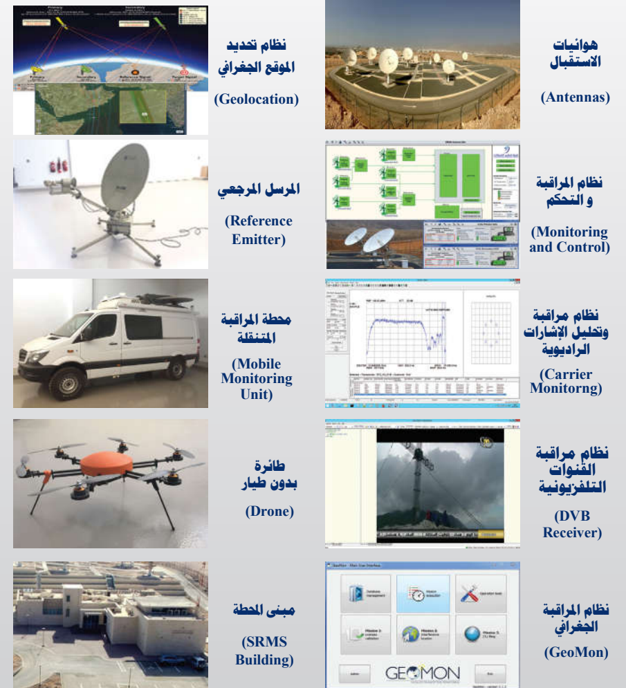
Figure 8: Main components of the Station
